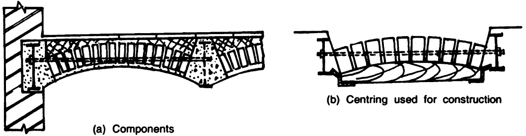
Fig. 21.1 Floor construction by jack arches with rolled steel joists and brick arches.
